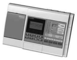
The VESDA VLP detector is the central element of the VESDA ASD product range. Using unique detection principles, the VLP has an alarm sensitivity range of 0.0015%– 6.25% obscuration/ft (0.005%–20% obscuration/m). The VLP is classed as a "Very Early Warning Smoke Detector". This means that it detects fire at the earliest possible stage and reliably measures very low to extremely high concentrations of smoke.
